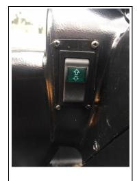
With this switch, the vehicle can be put in forward and rearward motion. The display indicates 'F' when in Forward, 'N' when in Neutral and 'R' when in reverse.
