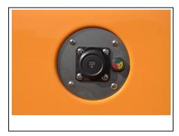
To charge the vehicle insert the designated charger into the socket in the vehicle. Then insert the connector into a 220V power outlet. It takes approximately 4 hours to charge an entirely empty battery. The red light will flash at the charging socket and turns green when fully charged.
